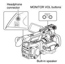
With the headphones connected to the headphone jack, the built-in speaker is turned off.
